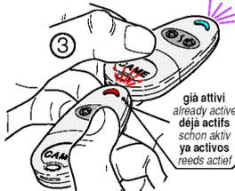
4. While the two remotes are against each other on the **working** remote press the left or right button depending on which button you pressed in step 2. I.e. if you pressed the left button on the **new** remote in step 2, press the left button on the **working** remote now. The light on the **new** remote should flash three times to confirm the programming was successful.
