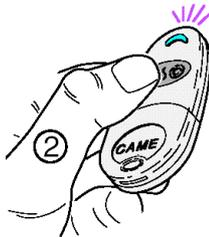
3. Now take the **working** remote and put the top of the remote against the “CAME” emblem on the **new** remote. NOTE: the two remotes must not be more than 1 inch apart!
