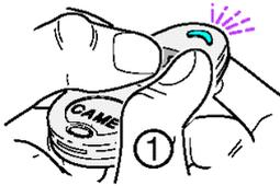
2. Still working on the **new** remote press and release the button that you would normally use to open your gate, i.e. if you use your left button to open your gate press and release the left button. The light should now stay illuminated.
